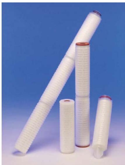
**PPC-A** filter cartridges are absolute rated, pleated polypropylene depth filters, they are equally suitable for use as membrane pre-filters or final polishing filters in applications that do not require membrane filtration.
